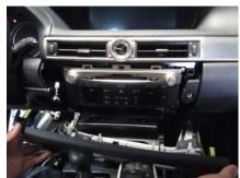
Remove the 2 x10mm nut. 1 on each side, bottom left and bottom right corner.
