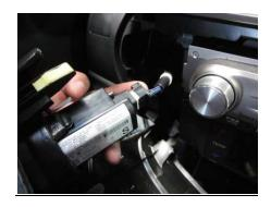
Route the push button switch wire to the side of the radio to your desired location. We chose to place it right under the parking brake lever (NT Series switch shown on the right)
