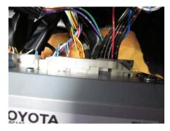
We picked the side of the radio to ground the wire.
