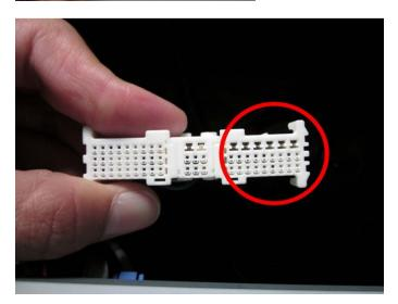
Connect the male side of the BB6223 connector to the female connector which was disconnected from the previous step. Make sure the connection is secure and that none of the pins are exposed on the side.
