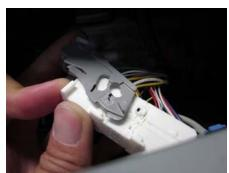
After the gray bracket is removed, the connector should look like this. The right side of the connector is what you need to disconnect from the main connector.
