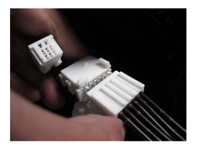
Using the supplied urethane insulation tape, tear off a size to cover the 2, 24 pin connectors that are mated to each other as shown on the right.
