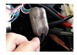
Take the female side of the BB6223 connector and link it back to the main connector, then mount the gray bracket back to the main connector.
